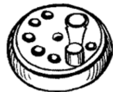
B. the 7 point switch
